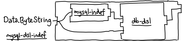
Figure 3. Composing libraries with requirements. It is possible to use components without filling all of their requirements; in that case, those requirements are propagated to the requirements of the enclosing component.
